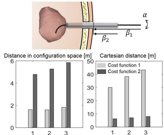
Fig. 1. Tubular aspiration robot (top) and mean traveled distance in configuration and Cartesian space for 3 patient datasets (bottom).
