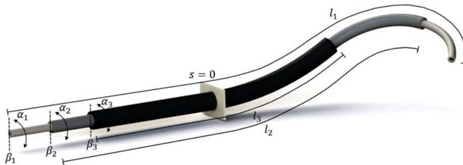
Figure 2: Tubular continuum manipulator composed of three tubes with tube length  $l_1, l_2, l_3$ , translational parameters  $\beta_1, \beta_2, \beta_3$  and rotational parameters  $\alpha_1, \alpha_2, \alpha_3$ .
