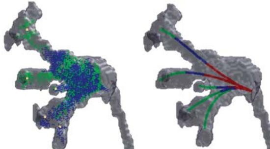
Figure 5: 10000 configuration samples for each of the 2 optimized tube sets for patient 1 marked as blue and green dots (left). Goal positions are marked as yellow dots. Example manipulator configurations reaching the goal positions (right).
