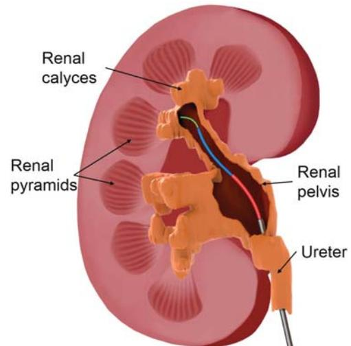
Figure 1: Tubular Manipulator composed of three tubes (red, blue, green) within the kidney extending out of an endoscope (gray).
